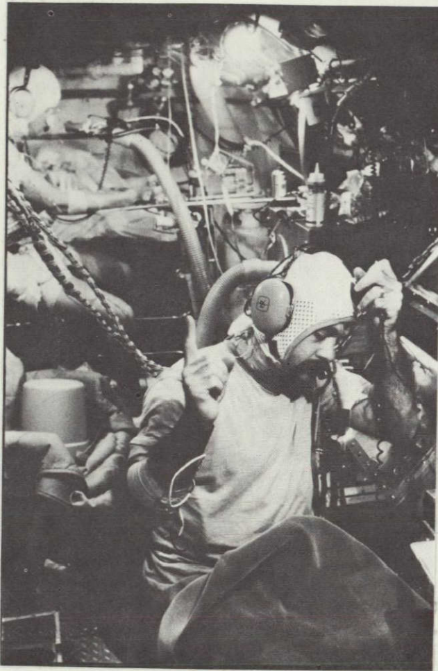
FIG. 6. Subject FS performing bone conduction audiometry on excursion to 1600-fsw pressure equivalent, signaling to controlling external investigator that sound is heard. Ergometer system in background. Somatosensory evoked response being elicited in Subject GM.
