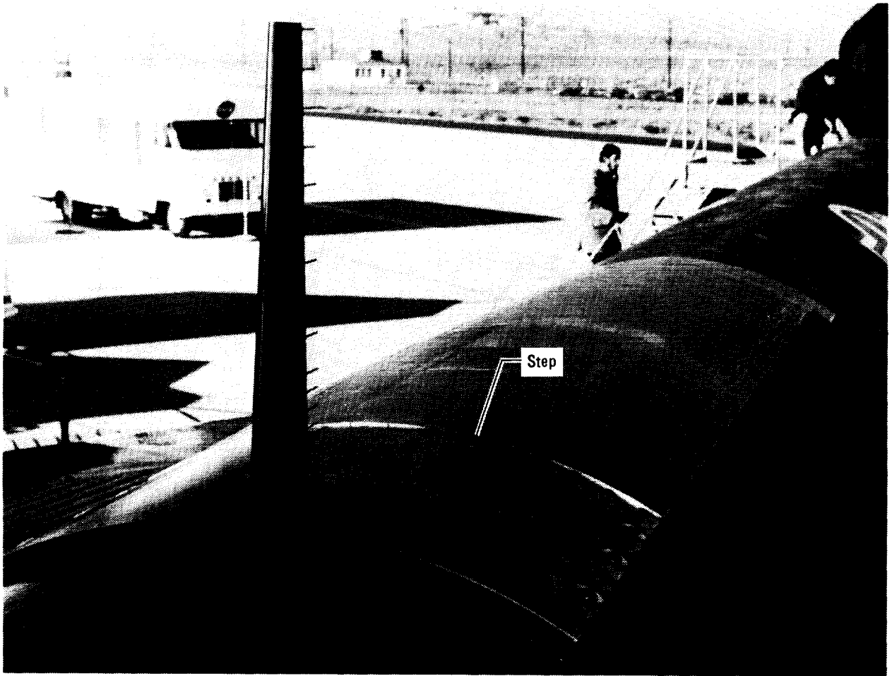
(b) Experiment viewed from rear. The boundary layer complex is in the aft location and the step height is 0.63 centimeter.
