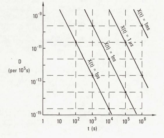
Figure 3. Largest allowable frequency drift coefficient, D, as a function of time, t, after perfect synchronization. The achievable time accuracy, X(t), is the parameter. D is used as a fractional frequency drift per 10<sup>5</sup> sec (approx. 1 day).
