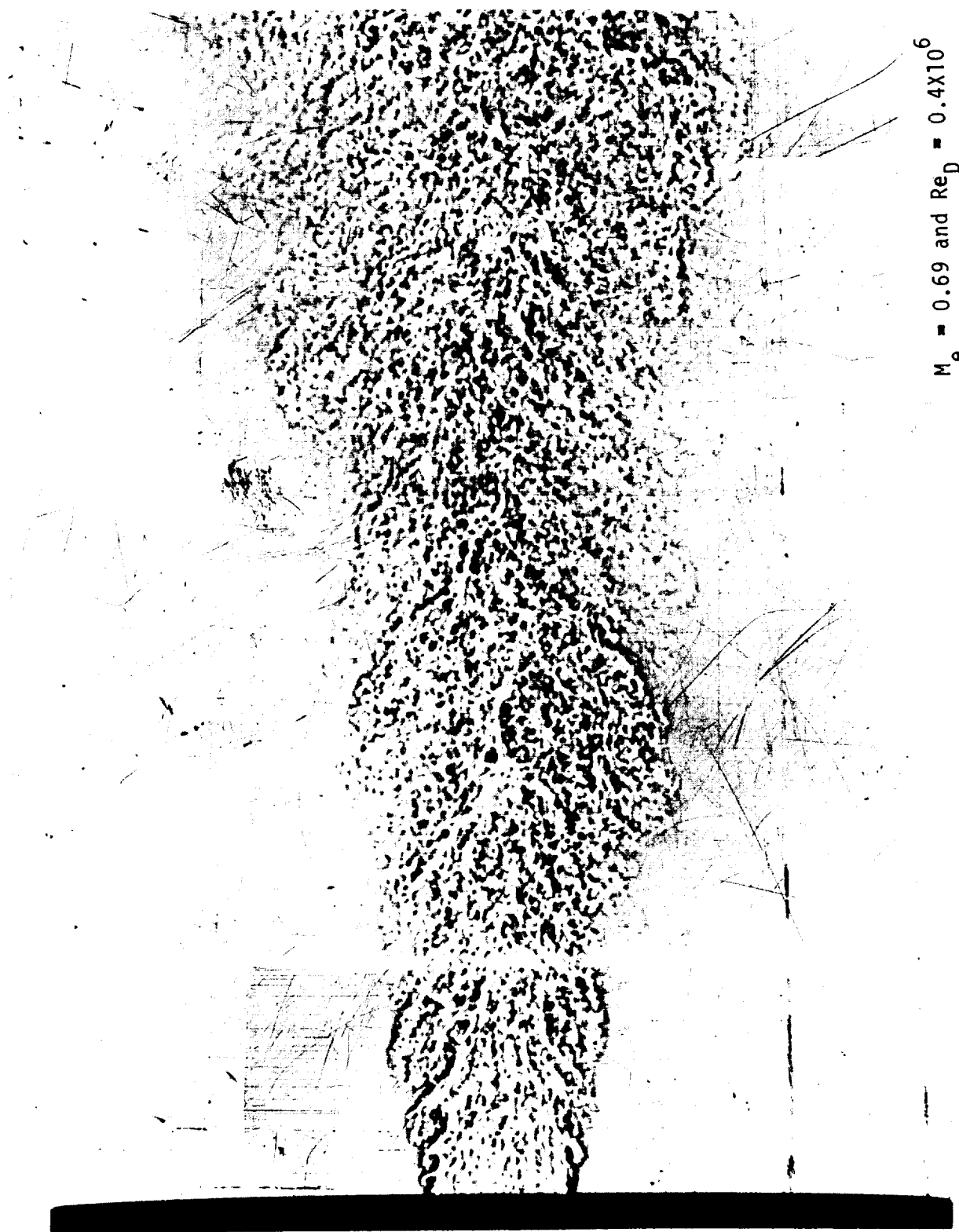
Figure 2. Shadowgraph showing large-scale turbulent structures.
