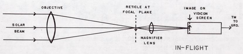
Figure 5. Rocket aspect system and co-alignment technique to be used on SIX
