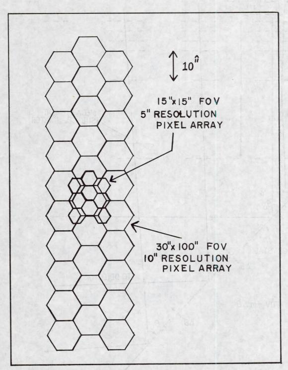
Figure 2 . The two stage nested MECA approach for the SIX experiment. Random arrays of hexagonal holes in the collimator grids form hexagonal pixels on the solar disk. Spacing of the various pixel axes, by alignment within the collimator grid frames, forms a field of view with flat spatial sensitivity.
