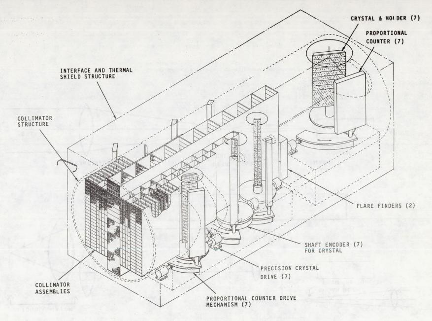
FIGURE 6.X-RAY IMAGING SPECTROMETER POLYCHROMATOR (XRISP) CONFIGURATION
