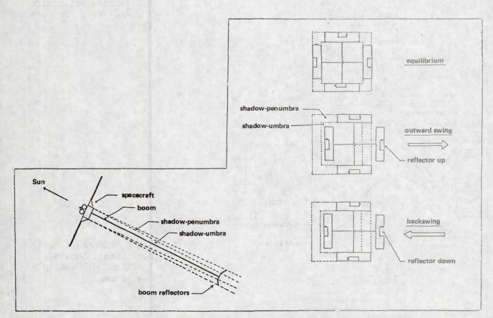
Figure 5. Passive Radiation Pressure Stabilizing Boom With Thermally-flexing Damping Reflectors.
