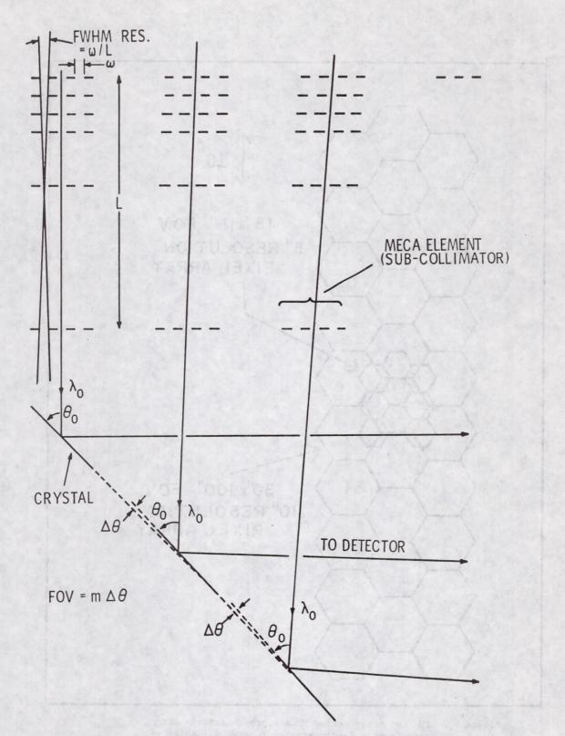
Figure 1. Multielement collimator array (MECA) concept. Collimation in one dimension is shown. Each subcollimator admits a pencil beam to its crystal and detector unit. Various subcollimator-crystal-detector units are offset from one another by  $\Delta\theta$  to provide imaging in pixels.
