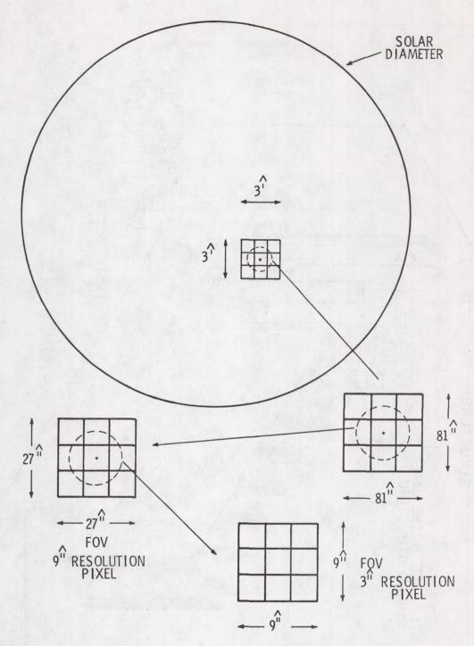
Figure 3. Imaging approach by means of nested MECA's. Nine pixels in the smallest field of view (FOV) just fill the central pixel of the next larger FOV. As the FOV increases from 9" to 180" the imaging resembles a telescope whose resolution degrades off-axis.
