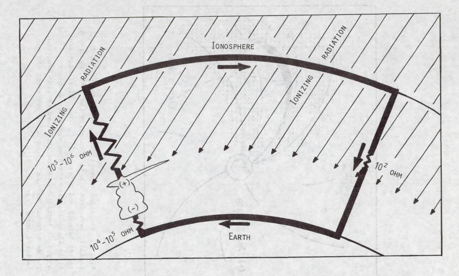
Fig. 2. Schematic of the global atmospheric electrical circuit illustrating relationships between resistive elements and showing accessibility of controlling resistive element above the thunderstorm generator to the varying component of ionizing radiation (after Markson (24)).
