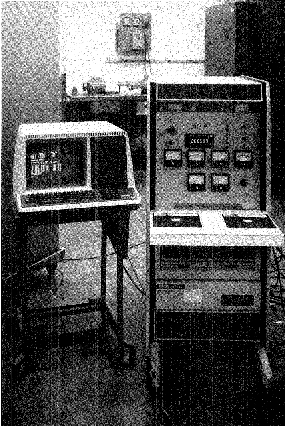
Fig. 3 CCAD Balancing Rig - Data Acquisition and Balancing System
