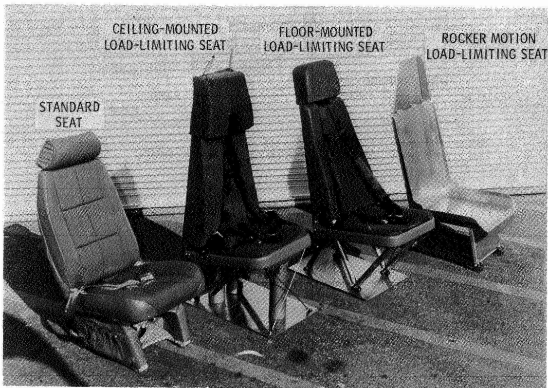
Figure 15.- Load-limiting seat concepts.
