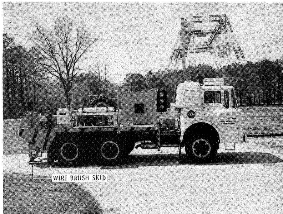
Figure 8.- Instrumented ground vehicle as used for wire brush skid tests.
