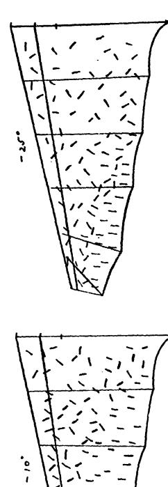
Figure 18,- Model 3 lower-surface tuft pattern.
