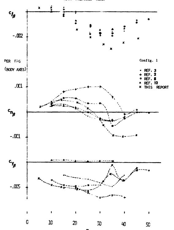
Figure 56.- Comparison of lateral data with previous work.
