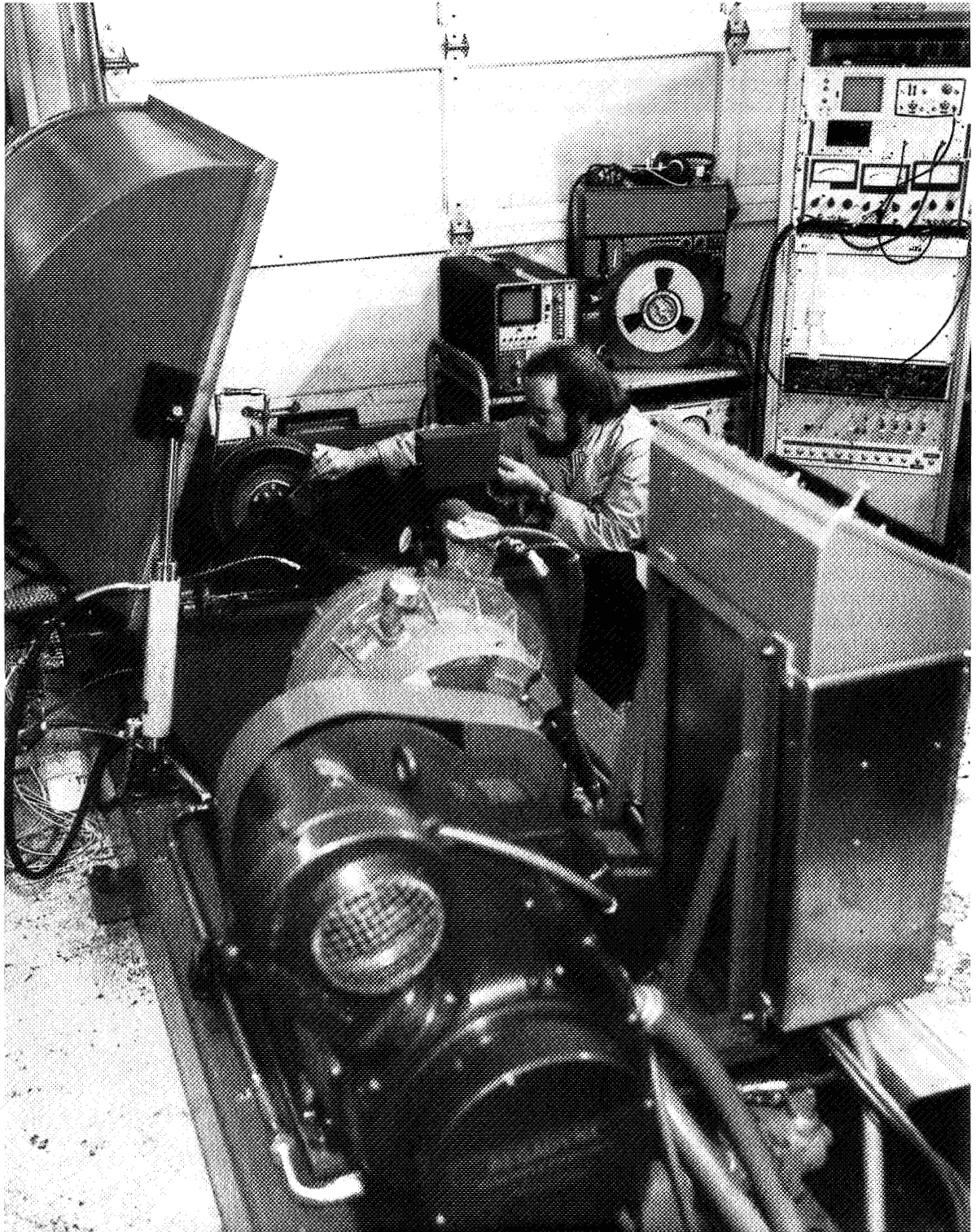
Fig. 168 CCAD Balancing Rig - Vacuum Chamber
