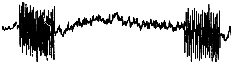
Figure 4. Gated 2.5 MHz surface wave pulses detected by wideband differential interferometry.
