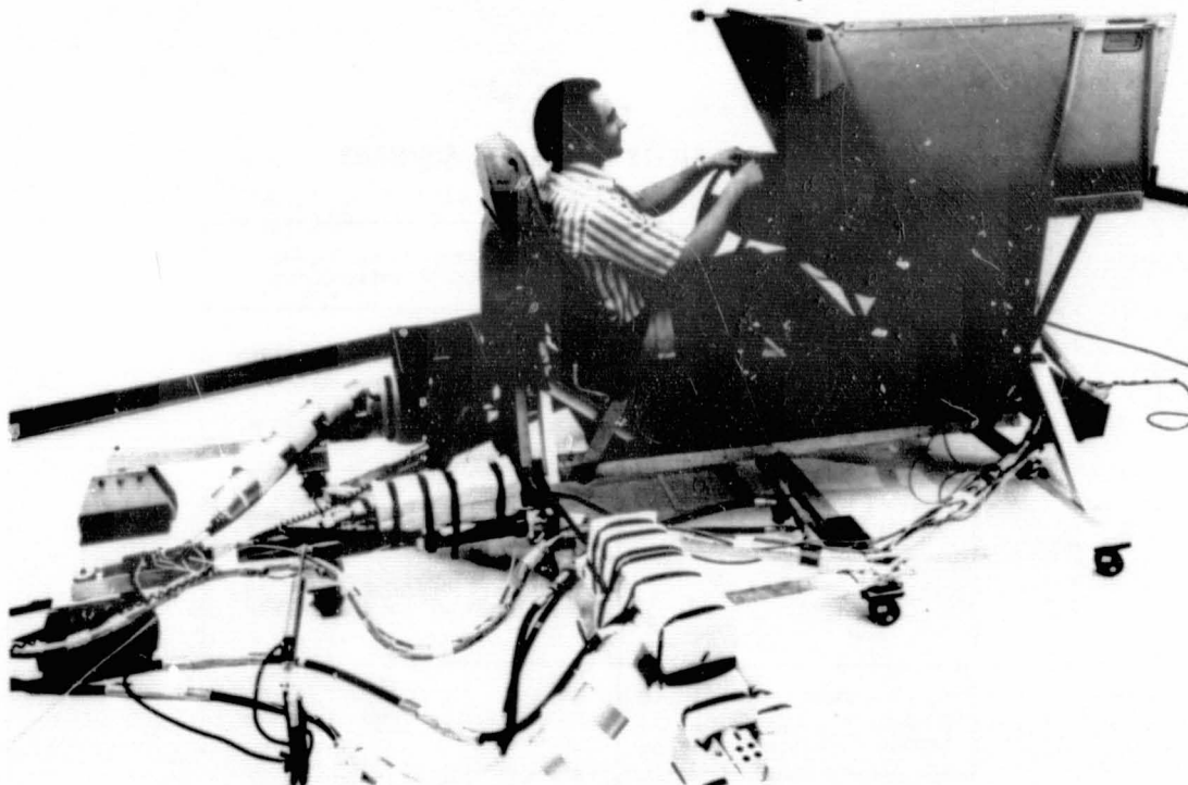
FIG. 2 DRIVING SIMULATOR MOTION PLATFORM
