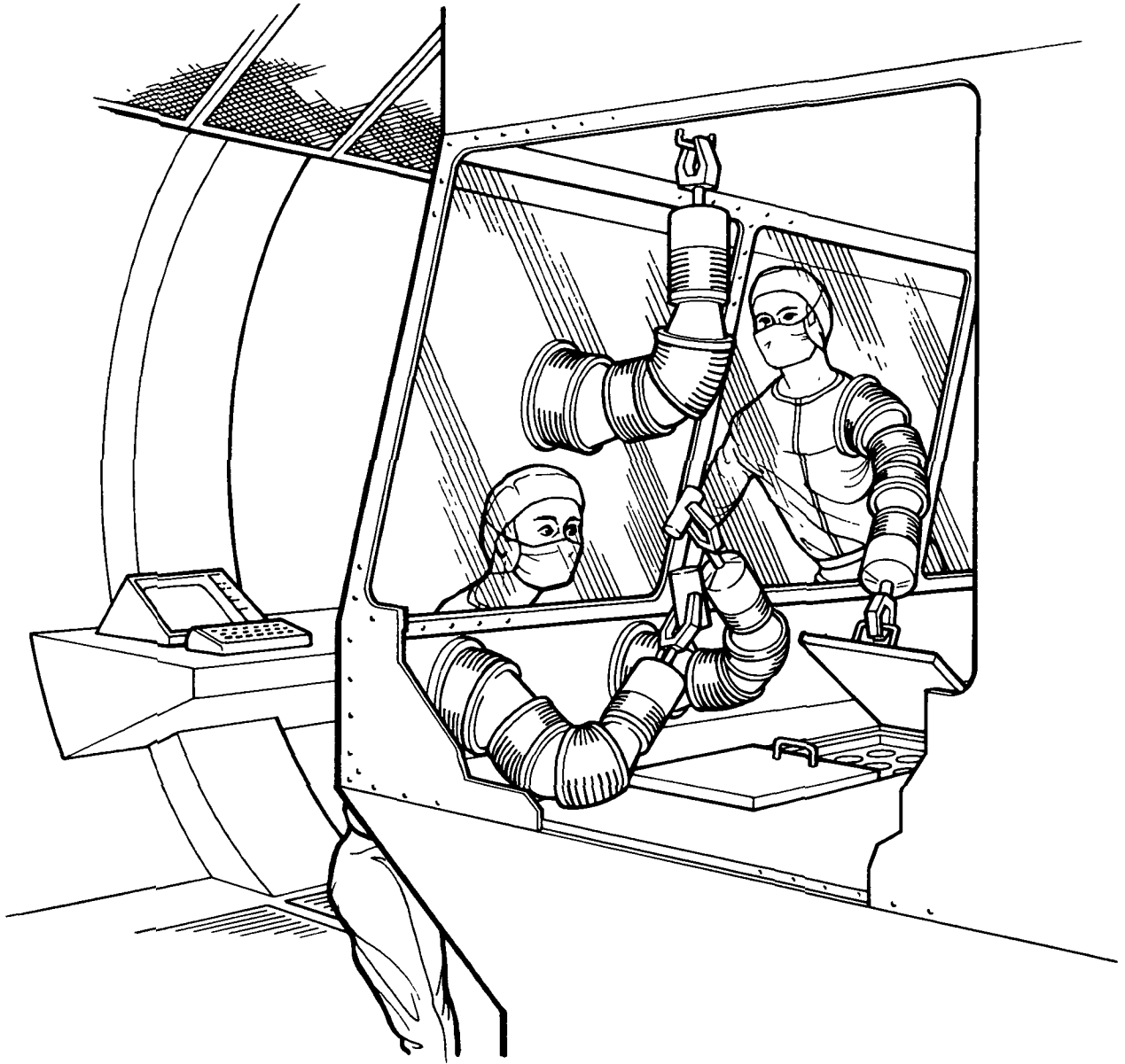
Figure 5-1. —A section of the biocontainment cabinet line within which the protocol will be executed. Note that the interior is accessed only with stainless steel “gloves.”
