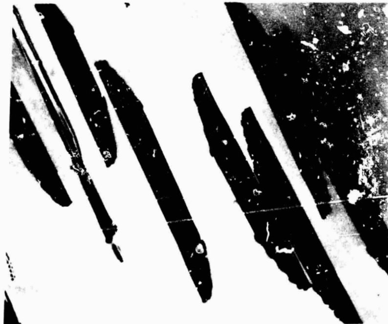
Fig. 7 Transmission electron micrograph of annealed abrasion damage showing stacking faults.
