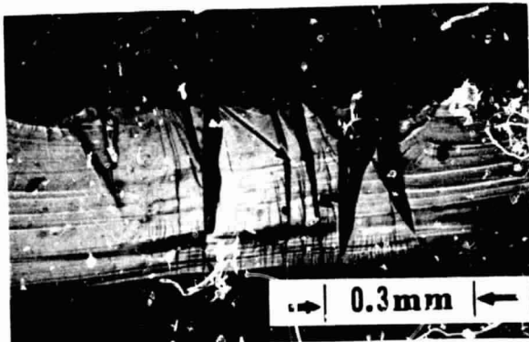
Fig. 3. Fracture surface of {100} exit chip. Direction of blade travel toward bottom of page.
