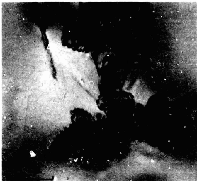
Fig. 2 Transmission electron micrograph of crack in silicon.
