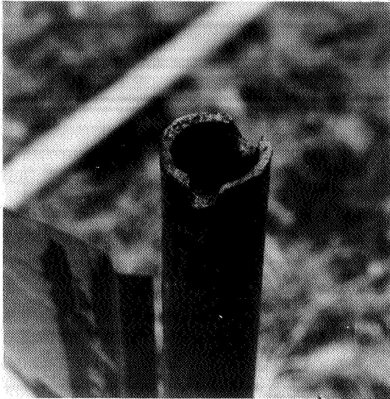
Figure 3 - Tail boom, Fatigue emanating from attachment holes.
