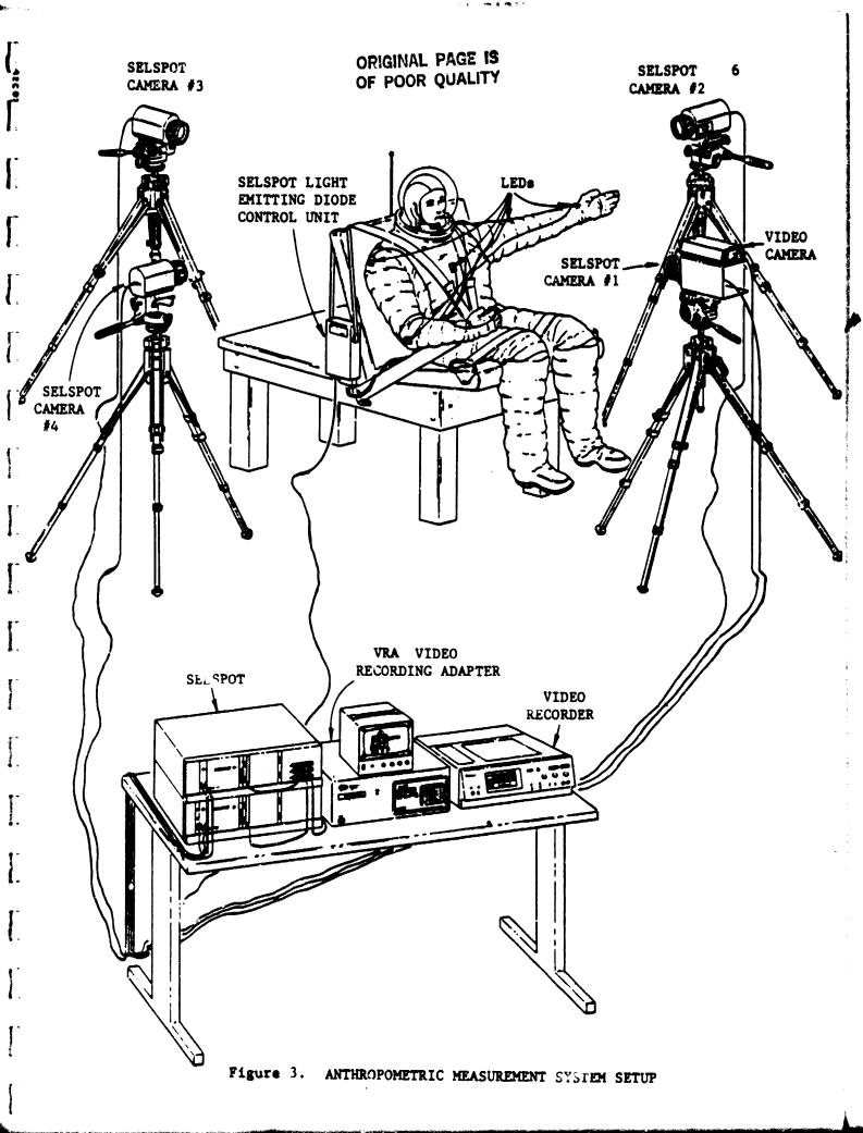
anthropometric data and experiment parameters are retrieved from the video signal. From this data, information such as the start time, date of the experiment, elapsed time into the experiment, and title of the test are obtained and decoded. The decoded information is then superimposed on the prerecorded television picture of the experiment.
