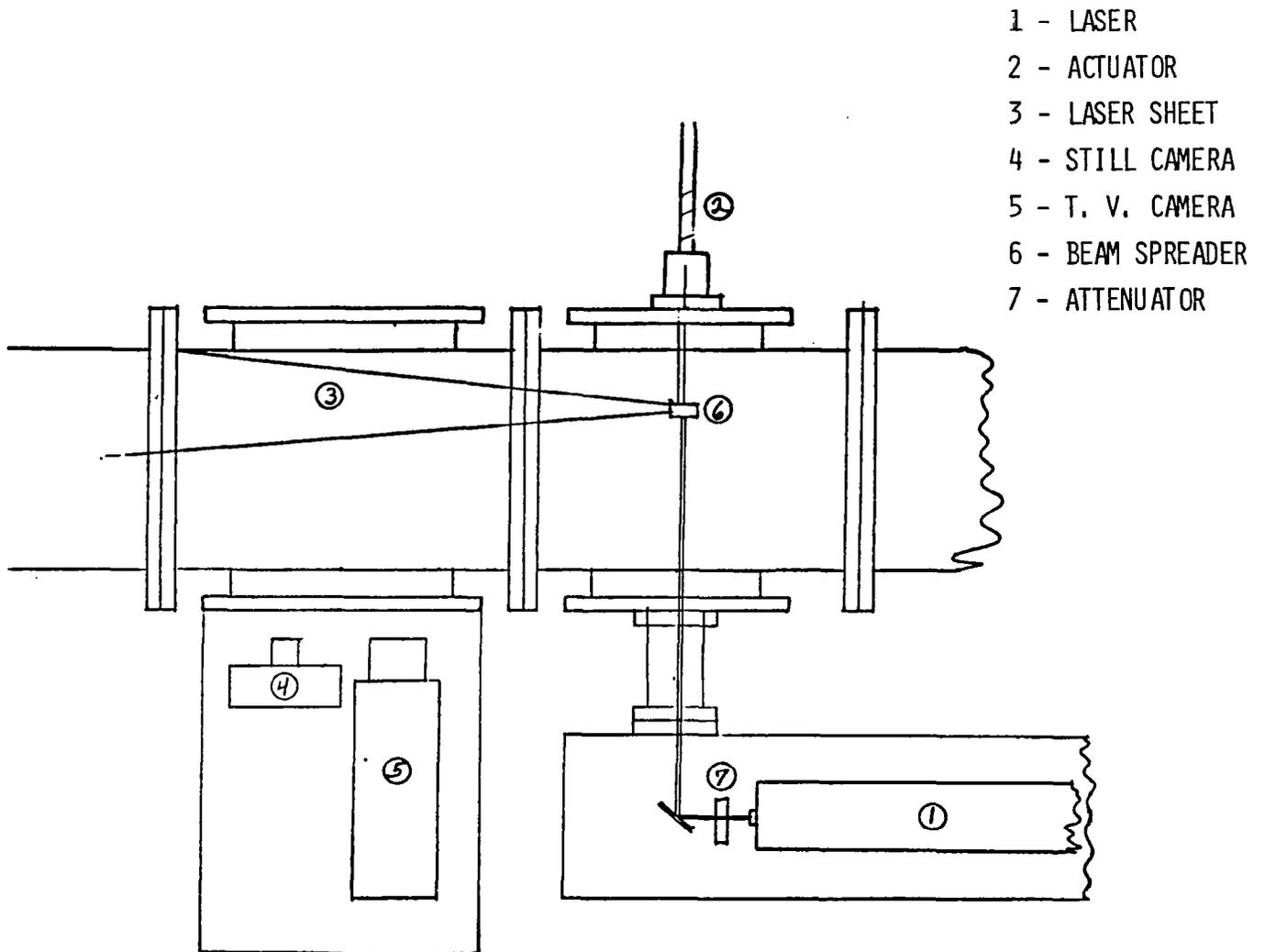
Figure 6. Laser Sheet Flow Visualization on Tunnel Centerline
