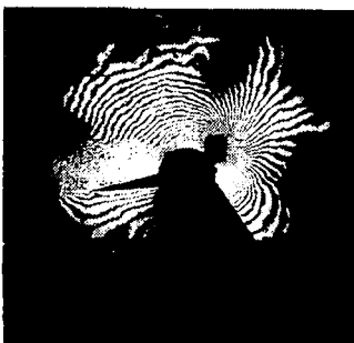
Figure 5.- Interferograms of 0012 airfoil undergoing dynamic stall.
