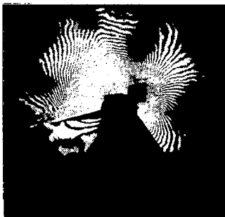
Figure 5.- Interferograms of 0012 airfoil undergoing dynamic stall.
