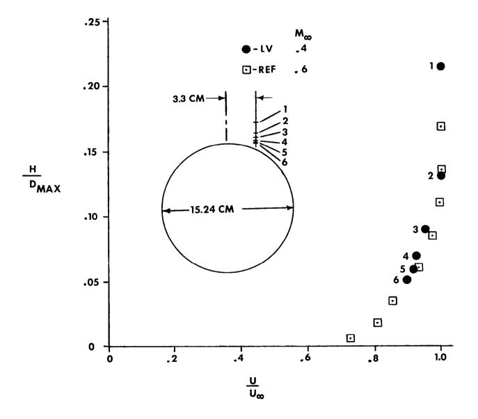
Figure 15.- Test results of vertical profile scan.
