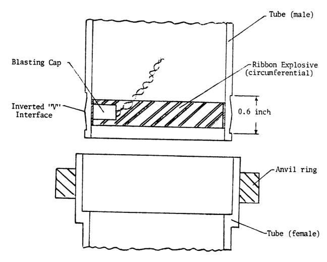
Figure 5.- Small-scale explosive seam welding setup for tubes.
