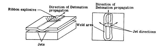
Figure 2.- Mechanisms involved in small-scale explosive seam welding process.
