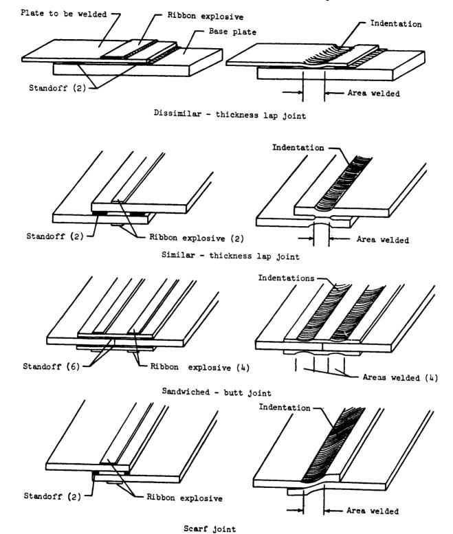
Figure 3.- Small-scale explosive seam welded joints.
