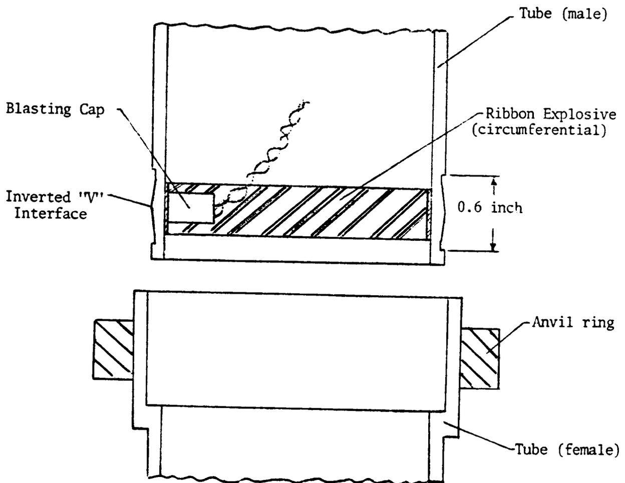
Figure 5.- Small-scale explosive seam welding setup for tubes.
