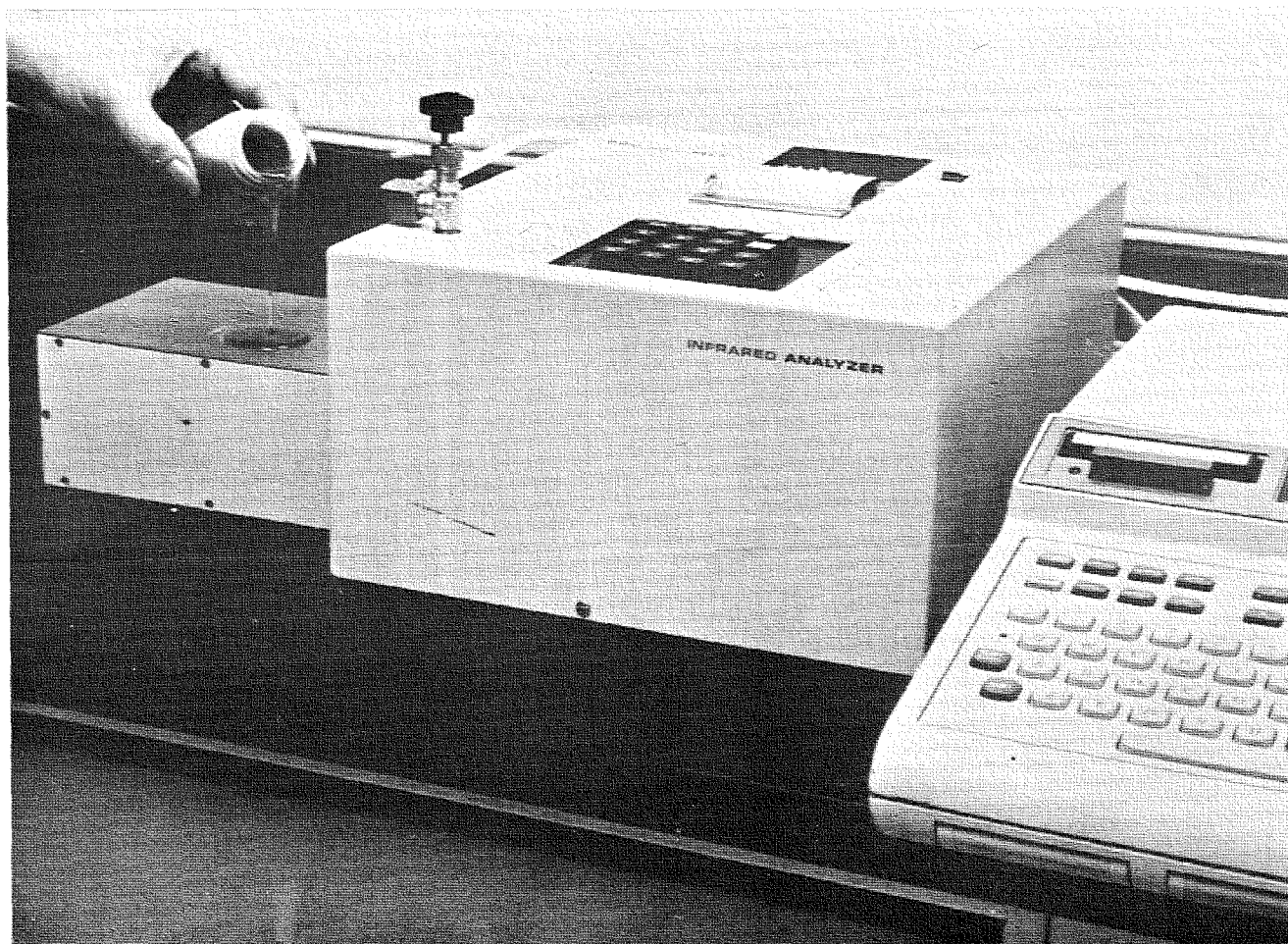
A Wilks Model 80 infrared spectrophotometer with MIR (multiple internal reflectance) sensing head. An H-P 9825 is interfaced to the instrument for use as a data logger and program controller. Oil samples are poured on the MIR for analysis, thereby eliminating the need for special sample preparation.
