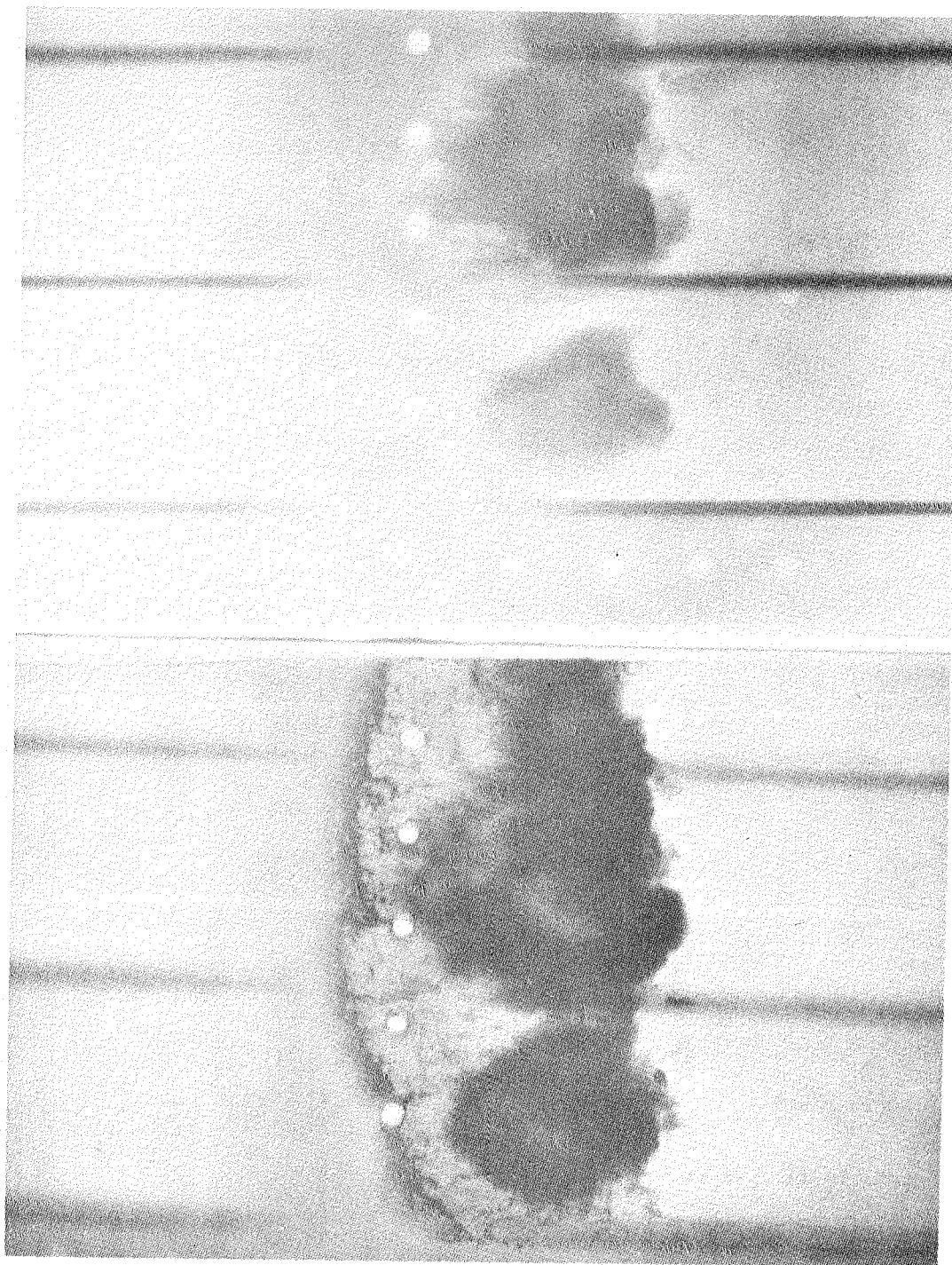
Figure 18. Neutron radiograph of C-130 wing structure. The neutron radiograph at the top is obtained in the usual way, and the one at the bottom with the use of a penetrant. The intergranular corrosion is seen to extend beyond the rivet holes, clearly explaining the cause of fuel leak from these holes.
