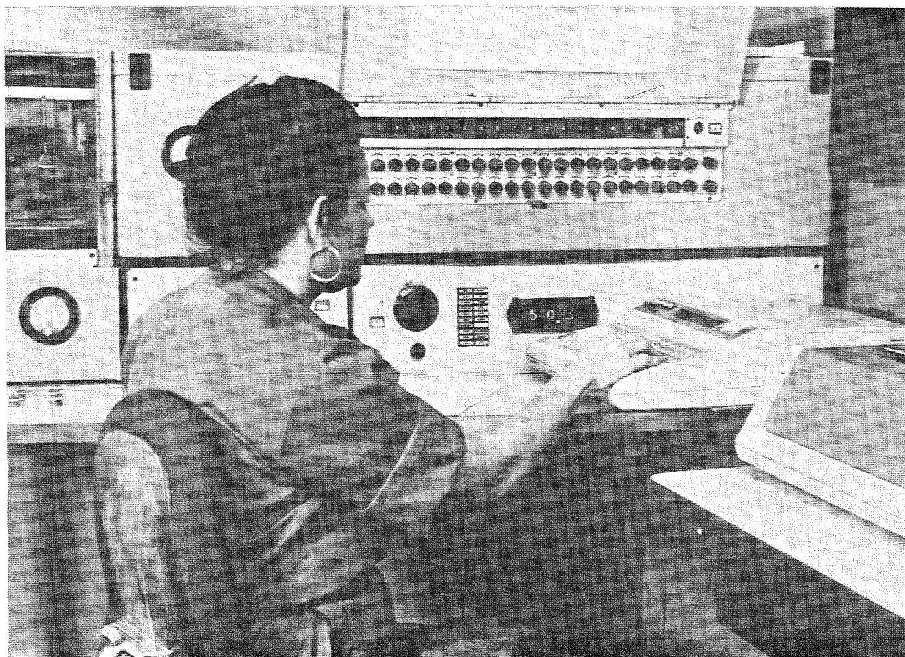
A Baird Corporation model FAS II atomic emission spectrometer interfaced to a Hewlett-Packard 9825 minicomputer. The H-P 9825 is used here as a data logger, recording analytical results on tape cartridges. These are in turn played through a central processing unit which updates the appropriate equipment files on a client's floppy disc.
