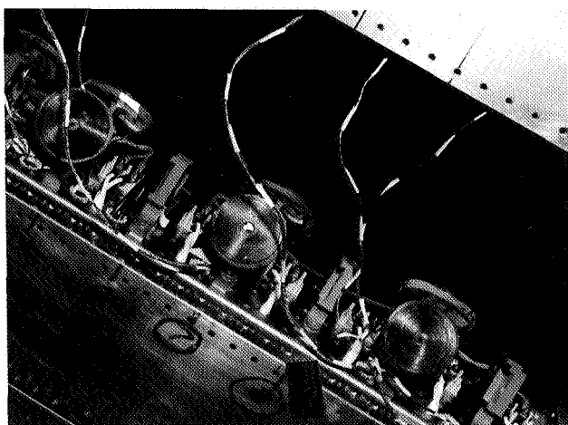
Figure 8. Closeup View of the Leading Edge of a Wing Section with the Electromagnetic Impulse System Installed
