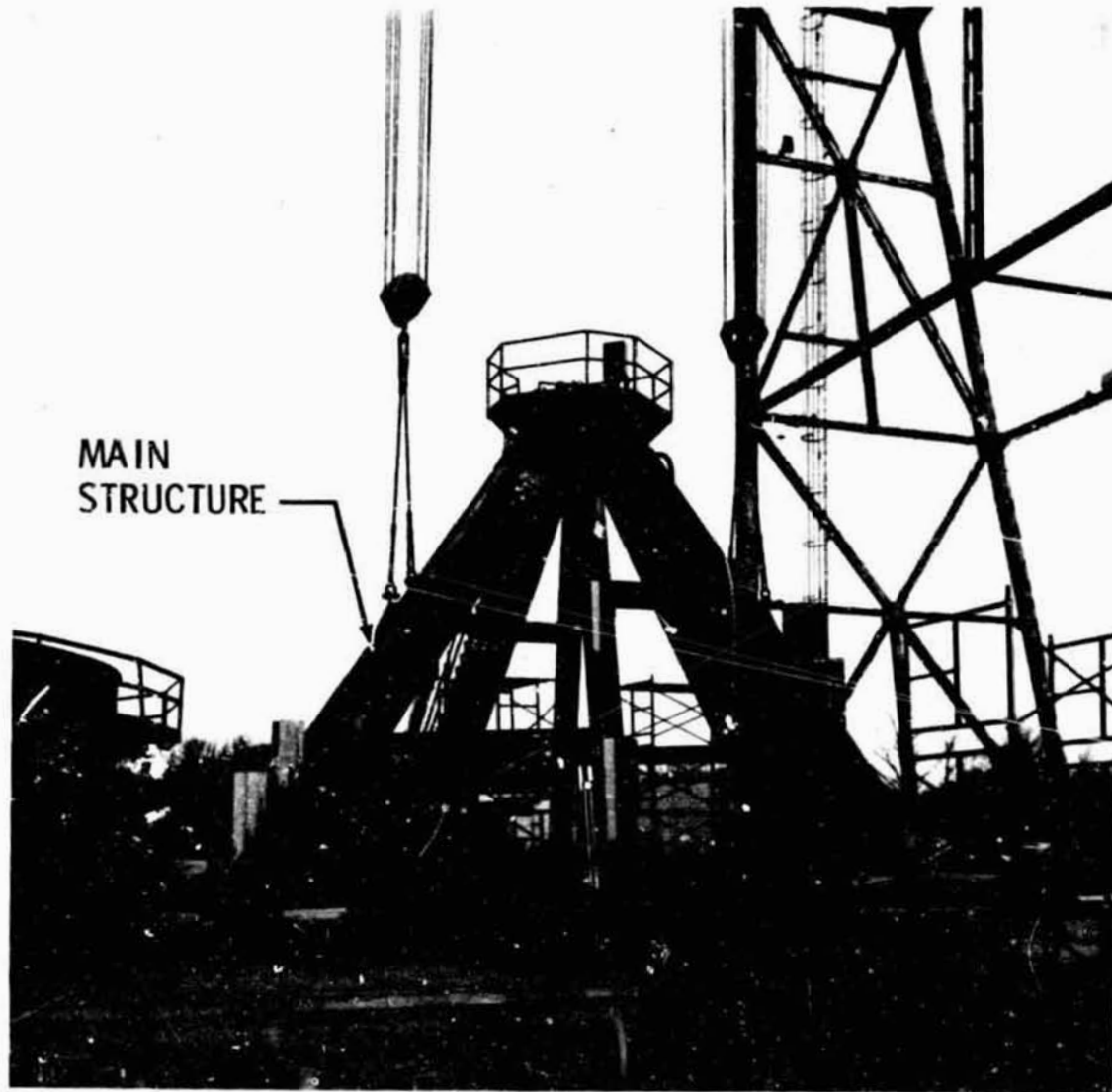
Figure 2. Thrust-Measuring System, Main Structure Pre-Installation
