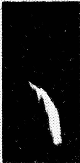
Figure 5. Frame and Streak Photographs of Laser Produced Plasmas at 2.0 Atmospheres in Hydrogen.
