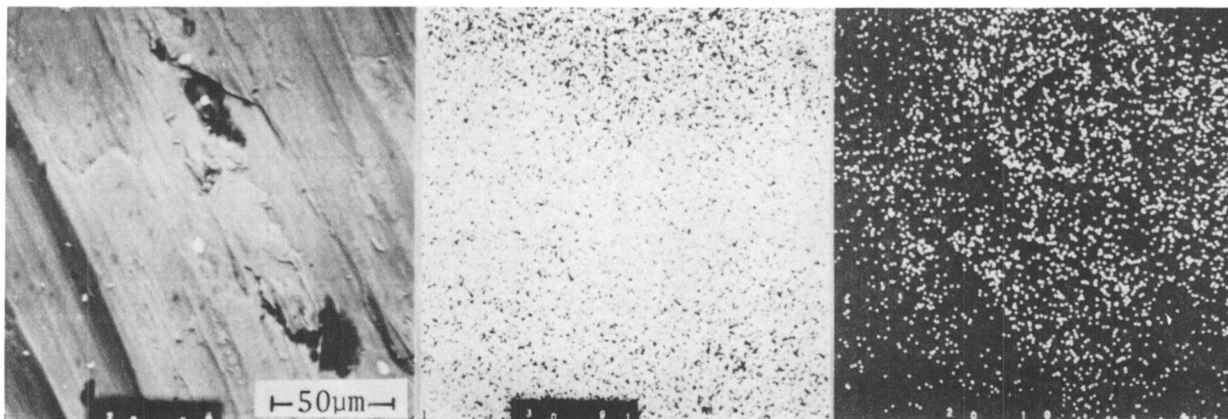
Back Scatter Electron Image. Cu K\alpha X-Ray Image. Ni K\alpha X-Ray Image.
