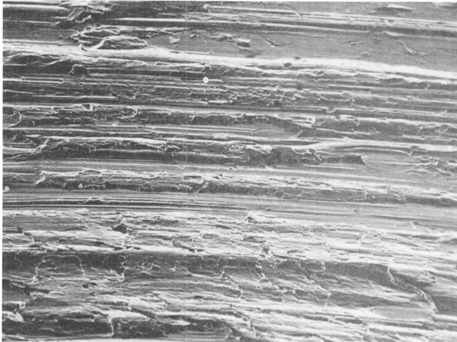
Fig. 14: Wear surface (C 60 steel, \sim 200 HV)
