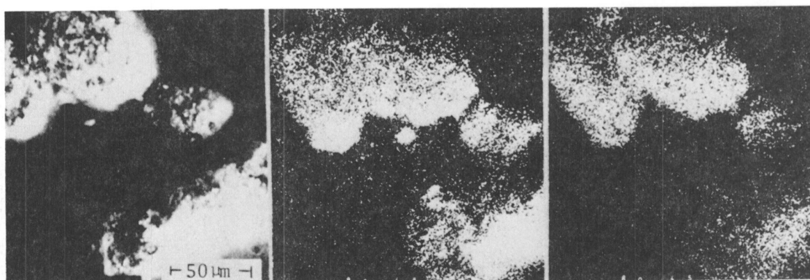
Secondary Electron Image. Si K\alpha X-Ray Image. Al K\alpha X-Ray Image. Figure 9. XMA PHOTOGRAPHS: Wear Particles Produced by SiC- Al_2O_3 Rubbing in Dry.
