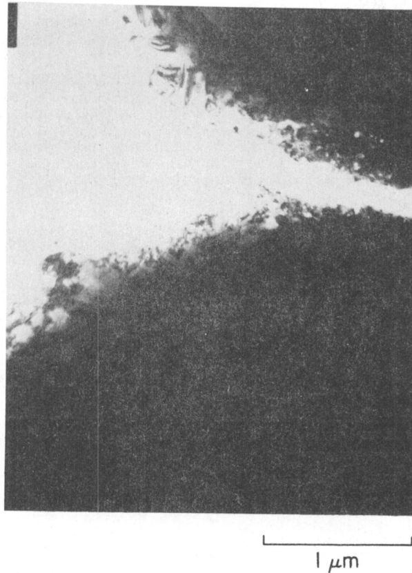
FIGURE 13. TEM MICROGRAPH OF A FOIL MADE FROM A SECTION THROUGH A WEAR SCAR ON COPPER-ALUMINUM SUBJECTED TO WEAR UNDER LUBRICATED CONDITIONS
