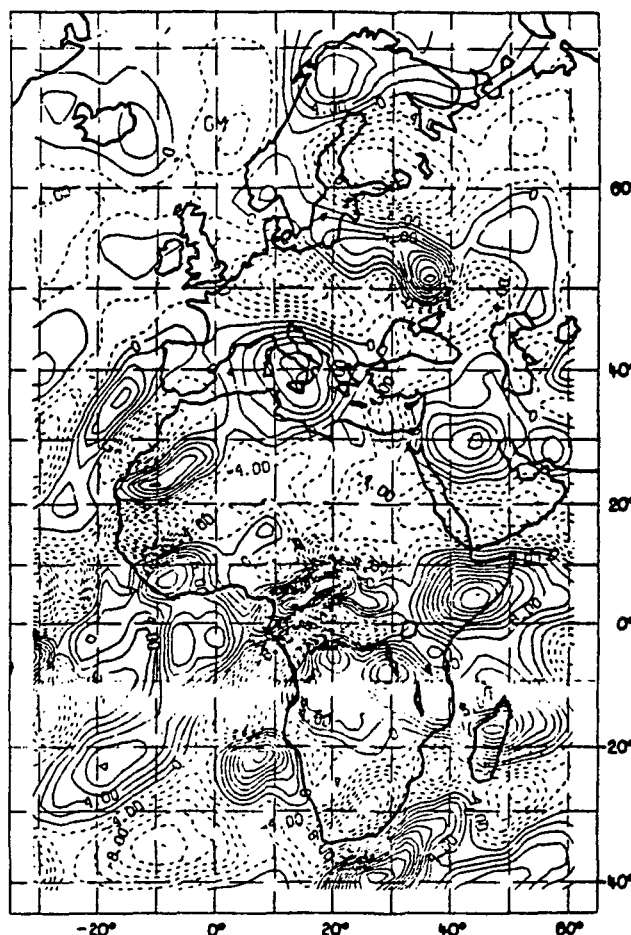
FIG. 2. Equivalent point source field approximation of 2^\circ -averaged scalar Magsat magnetic anomaly data differentially reduced to radial polarization at 400 km elevation. The normalized amplitude for the polarizing field is 60,000 nT. Contour interval is 2 nT.
