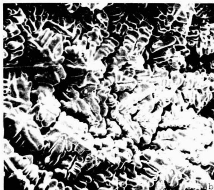
Views of transverse sections of porous dendritic networks of partially solidified Al-4%Si samples. (a) Stereo-photograph of a columnar network structure, x150; (b) SEM view of an equiaxed network structure, x22.
