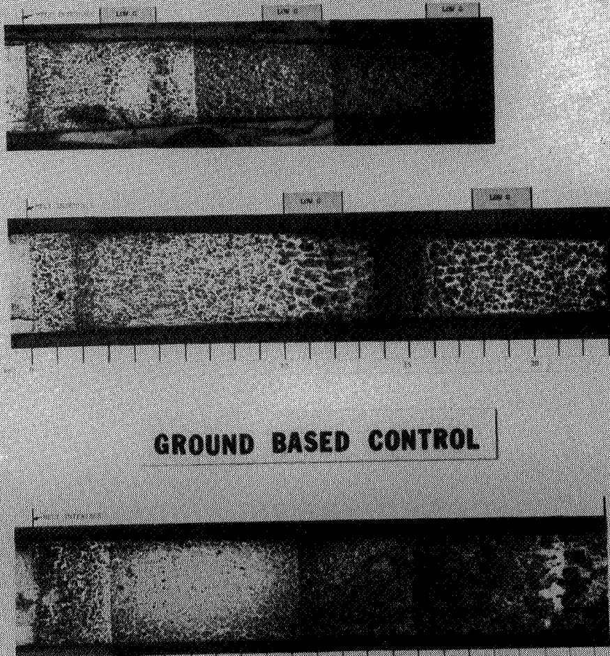
Figure 10. Low magnification (originally x 12) composite micrographs of high phosphorus hypereutectic flake graphite iron samples: bottom – ground-based sample; middle – flight sample; top – flight sample.
