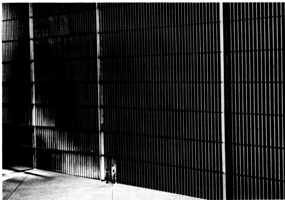
The size of the Ames 40- by 80-foot full-scale wind tunnel is evident in these two internal photographs. Above, an automobile parked inside the tunnel (above) is about the size of each of the six motors that power the airflow. A man stands beside one of the propeller blades of the lower left mount. Below, turning vanes in the tunnel tower over two workers on the tunnel floor. (ARC)
