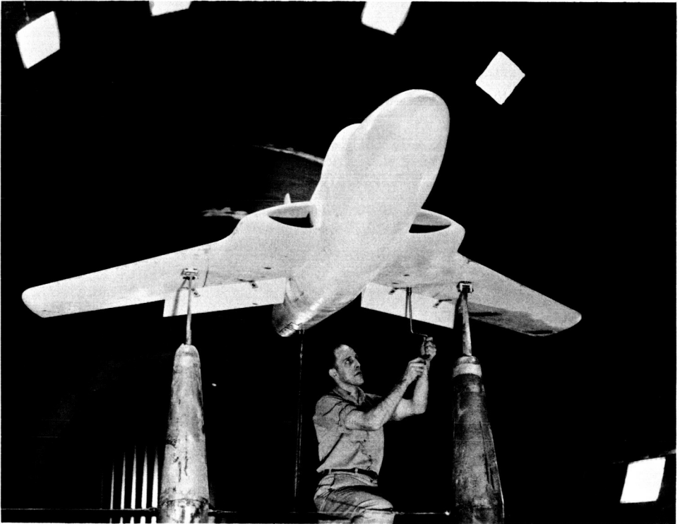
Above, a phantom drawing of the Langley 19-foot pressure tunnel shows the test section at the front center, the turning vanes at the four corners, and the drive fan at the left rear. The air moves clockwise. Below, a technician mounts a model of Republic Aviation's F94F in the test section. (LaRC)
