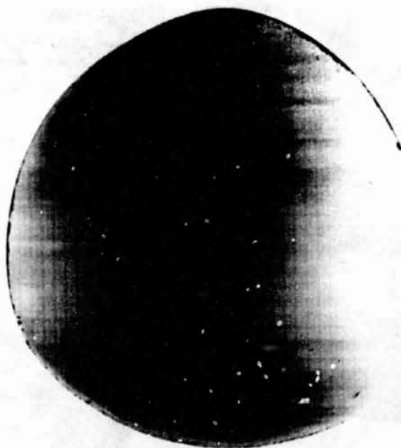
(220) transmission x-ray topograph of a dislocation-free 0.1 ohm-cm Ga-doped float-zoned silicon crystal wafer
