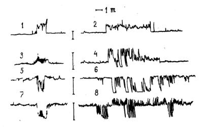
Fig. 1. Characteristic examples of radio emission bursts of near earth space and sudden short-time cosmic noise absorption (SCNA) detected at the frequency of 38 MHz. 1,2 - Sporadic bursts of overage power. 3 - Sporadic bursts with oscillating fine structure. 4 - Sporadic bursts with short-time cosmic noise absorptions. 5,67- Short-time sporadic of cosmic noise with oscillating fine structure. 8 - Series of sporadic absorptions of cosmic noise with oscillating fine structure.
