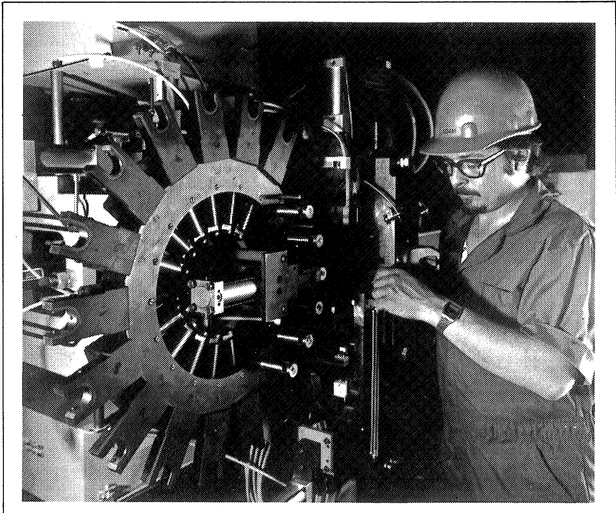
Figure 9. Automatic Tool Changer Holds 12 Drills and 6 Bucking Anvils.
