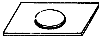
e. Lap Welding a Cover Plate to a Flat Plate
