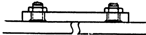
c. Stud weld bolts on the structure and then securely fasten the cover plate work holes by nuts
