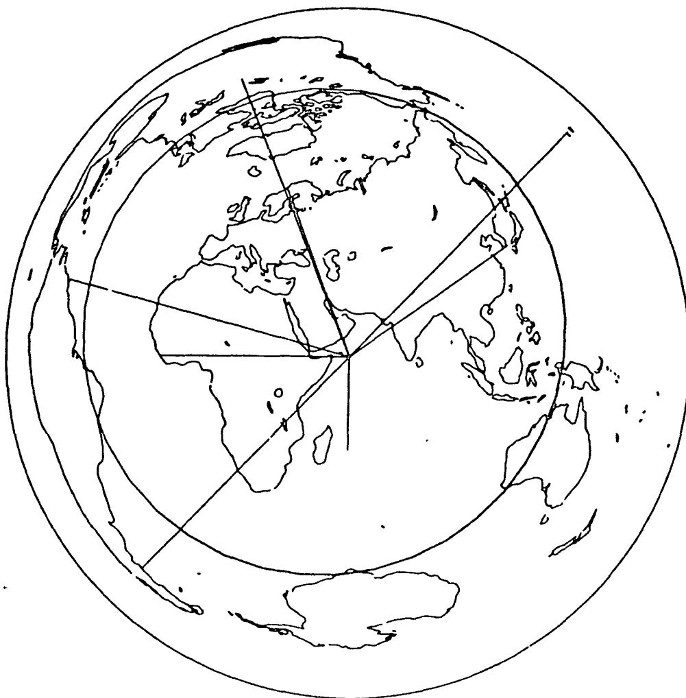
FIGURE 10 True azimuthal plot of sonde-omega transmitter geometry for representative drop in the Arabian Sea. Great circle least-distance paths for all eight omega stations are shown. The circle represents the solar terminator at about 1300 LST.
