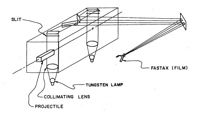
Figure 1. Diagram of Hall Station and Camera System.
