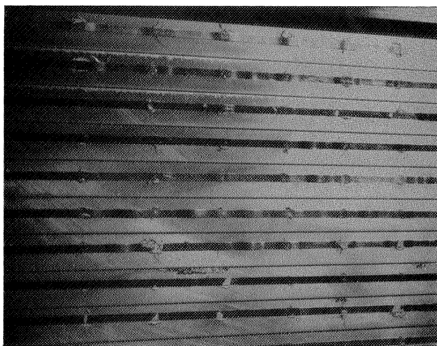
Back Side of Arco Test Module Showing Added Conductive Ribbon Attached with Conductive Epoxy
