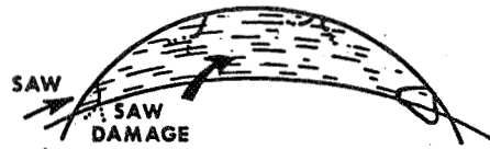
B. SLICING PUTS IN SAW DAMAGE AND CHIPS OUT SOME GRINDING CAVITIES.
