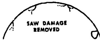
C. LAPPING, ETCHING AND POLISHING REMOVES SAW DAMAGE BUT NOT ALL OF THE GRINDING DAMAGE.
