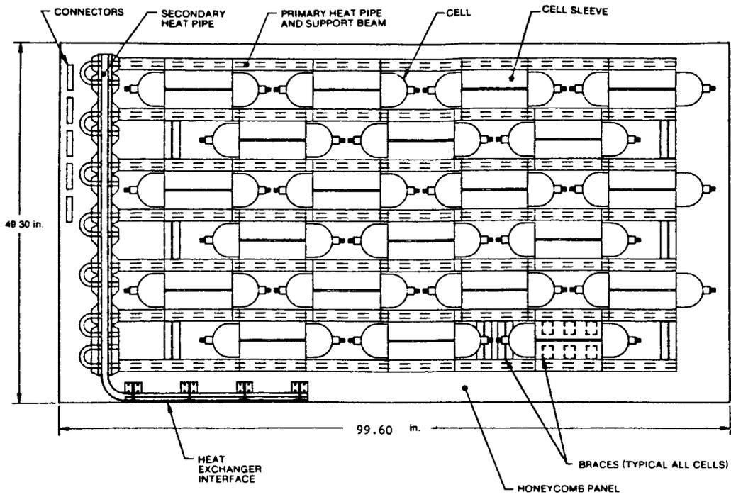
Figure 5. SPACE STATION NiH<sub>2</sub> BATTERY ASSEMBLY LAYOUT
