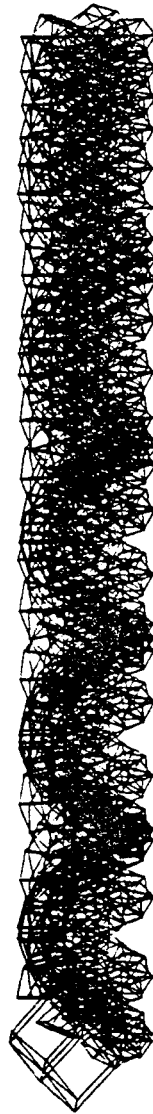
Fig. 5.10. Typical mode shape showing slipping between strands.
