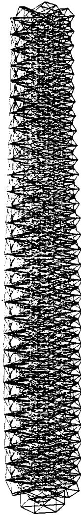
Fig. 5.9. Typical mode shape showing end separation (with end mass).
