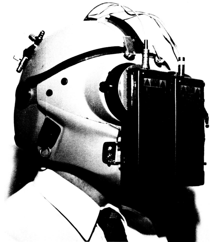
Two miniature monitors on a helmet-mounted platform provide a real-time window into a simulation scenario. The helmet positioning device allows a 360-degree field of vision. Slightly offset left and right images provide true depth of field. (Courtesy of Johnson Space Center.)
