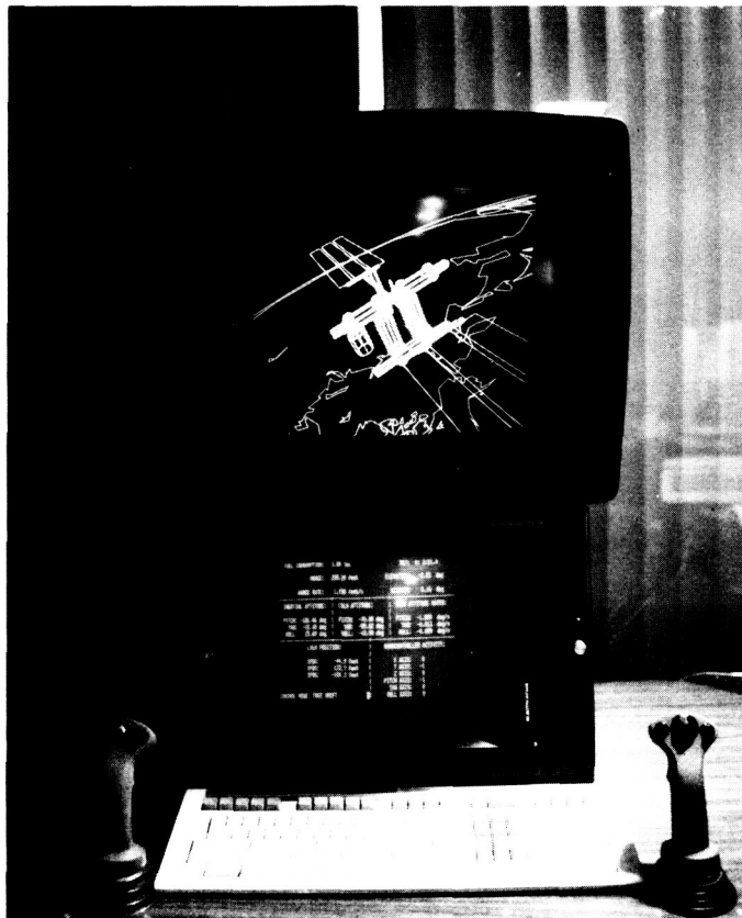
Advancements in automation technology will allow complex simulations to be performed on the ground and in space, in real time. This photograph shows a simulation of a spacecraft interacting with a Space Station. This workstation-based, real-time, man-in-the-loop simulation system is being used to investigate a variety of integrated space operations. (Courtesy of Johnson Space Center.)
