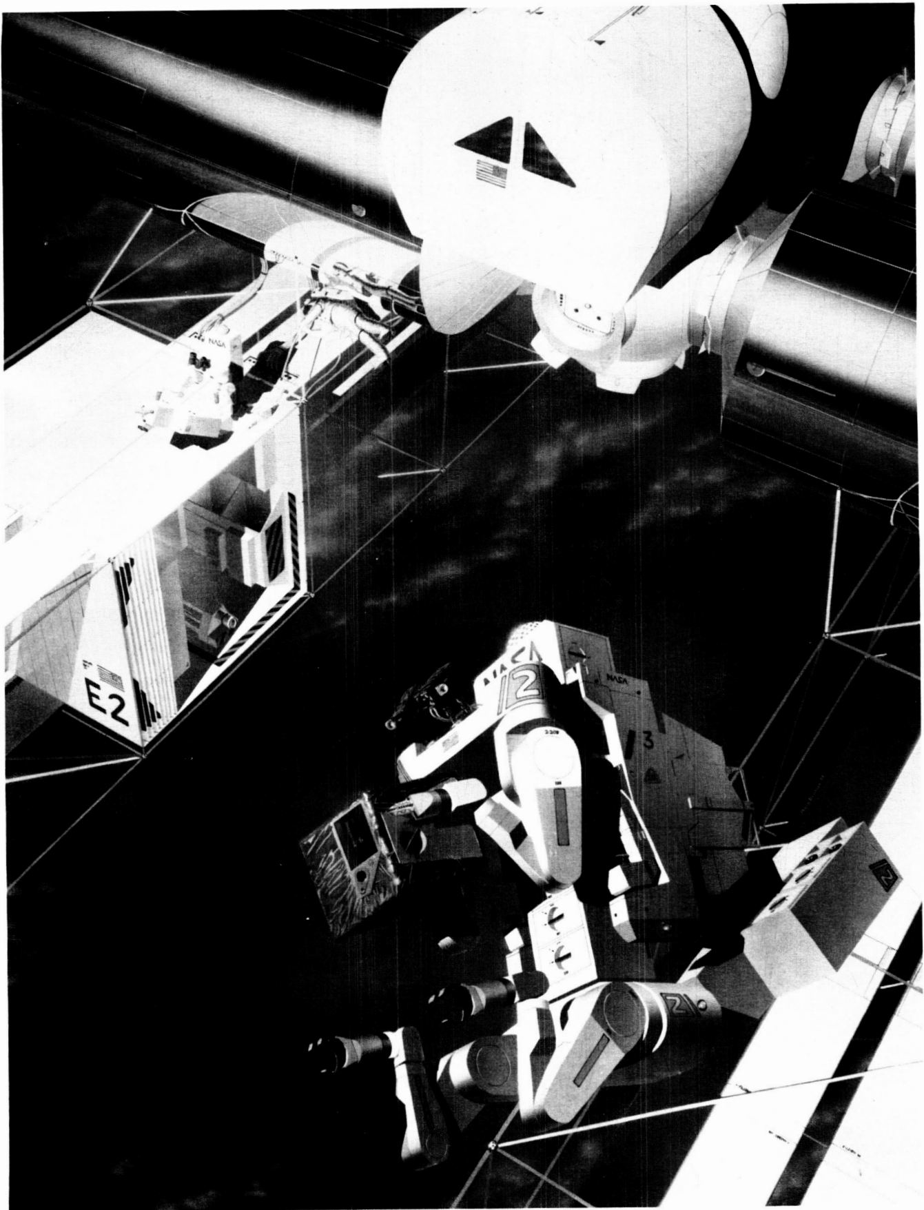
A generic robot can assist the crew in assembly, maintenance, servicing, deployment, retrieval, and transportation. This illustration depicts a robot changing out an orbital replaceable unit. (Courtesy of McDonnell Douglas.)
