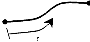
Figure 1 Hermite Spline Defining a Line
