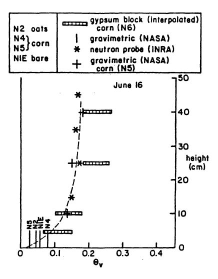
Fig. 4 Vertical distribution of volumetric soil moisture at Lubbon on 16 June 1986, as measured by gypsum blocks in fields N6 (corn) by neutron probe (asterisks) and by gravimetric sampling in field N5 (corn). The vertical bars at the bottom represent averages of 0-5 cm gravimetric water content samples in four fields. The dashed line suggests the mean vertical soil moisture profile.
