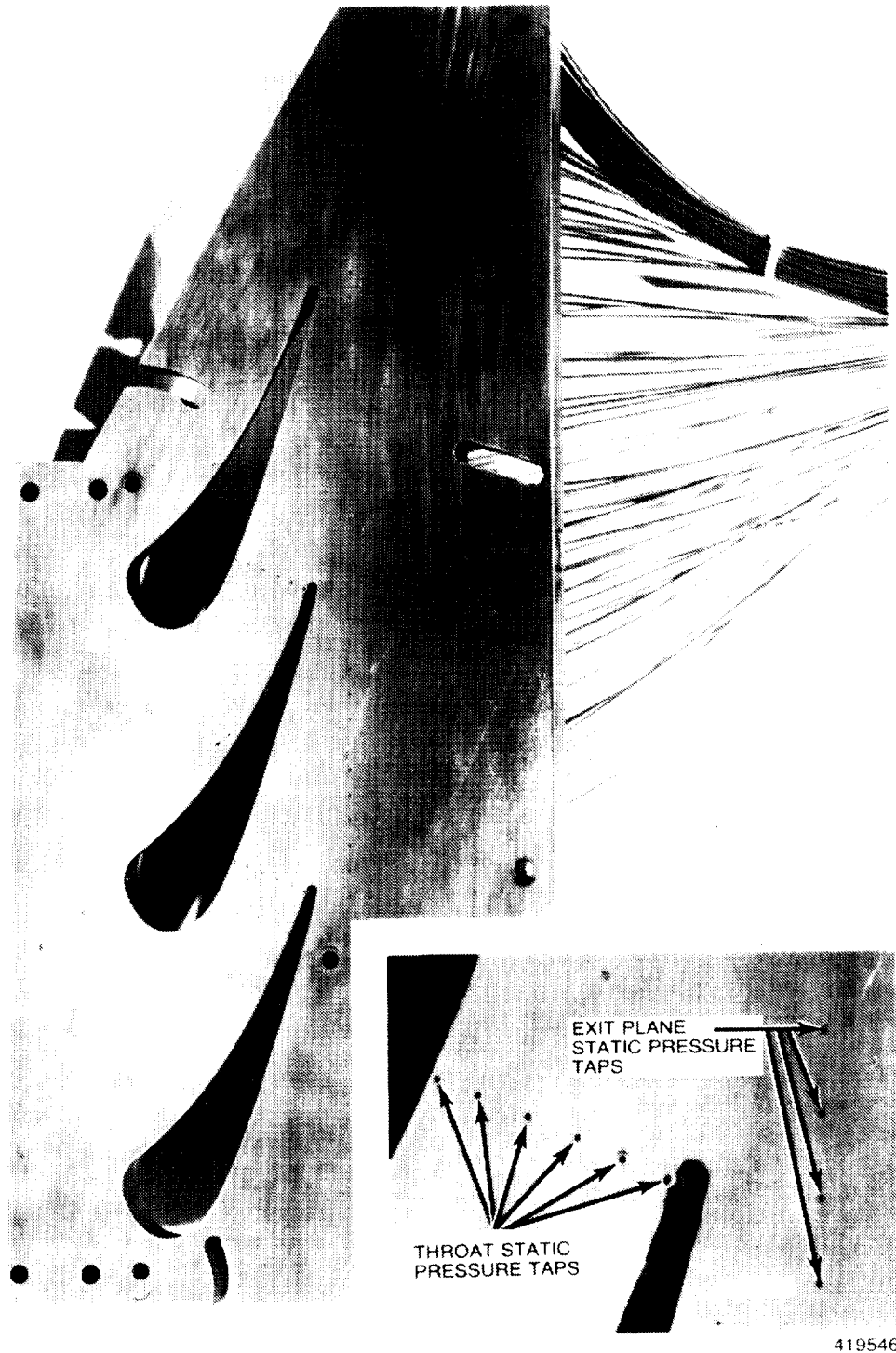
Figure 4. Details of the endwall static pressure taps at the exit plane and cascade throat.
