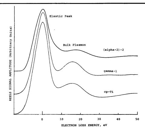
Fig. 3 The reflected electron energy loss spectrum for an uncharged alpha-2 alloy, gamma alloy, and cp-Ti. The first major peak measured from the main elastic peak is the bulk plasmon loss peak.
