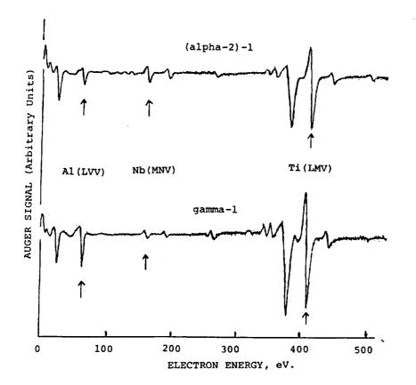
Fig. 1 AES spectra of the sputter cleaned surfaces of an uncharged representative alpha-2 and gamma titanium aluminide alloy.
