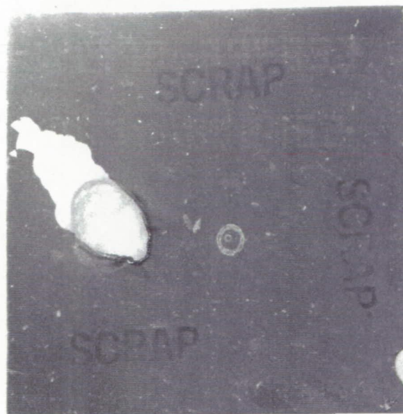
Figure 2. Low magnification OM photomicrograph of damaged tile surface. 0.5X
