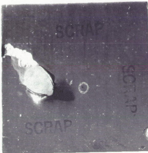
Figure 3. Low magnification OM photomicrograph of damaged tile surface. 0.5X
