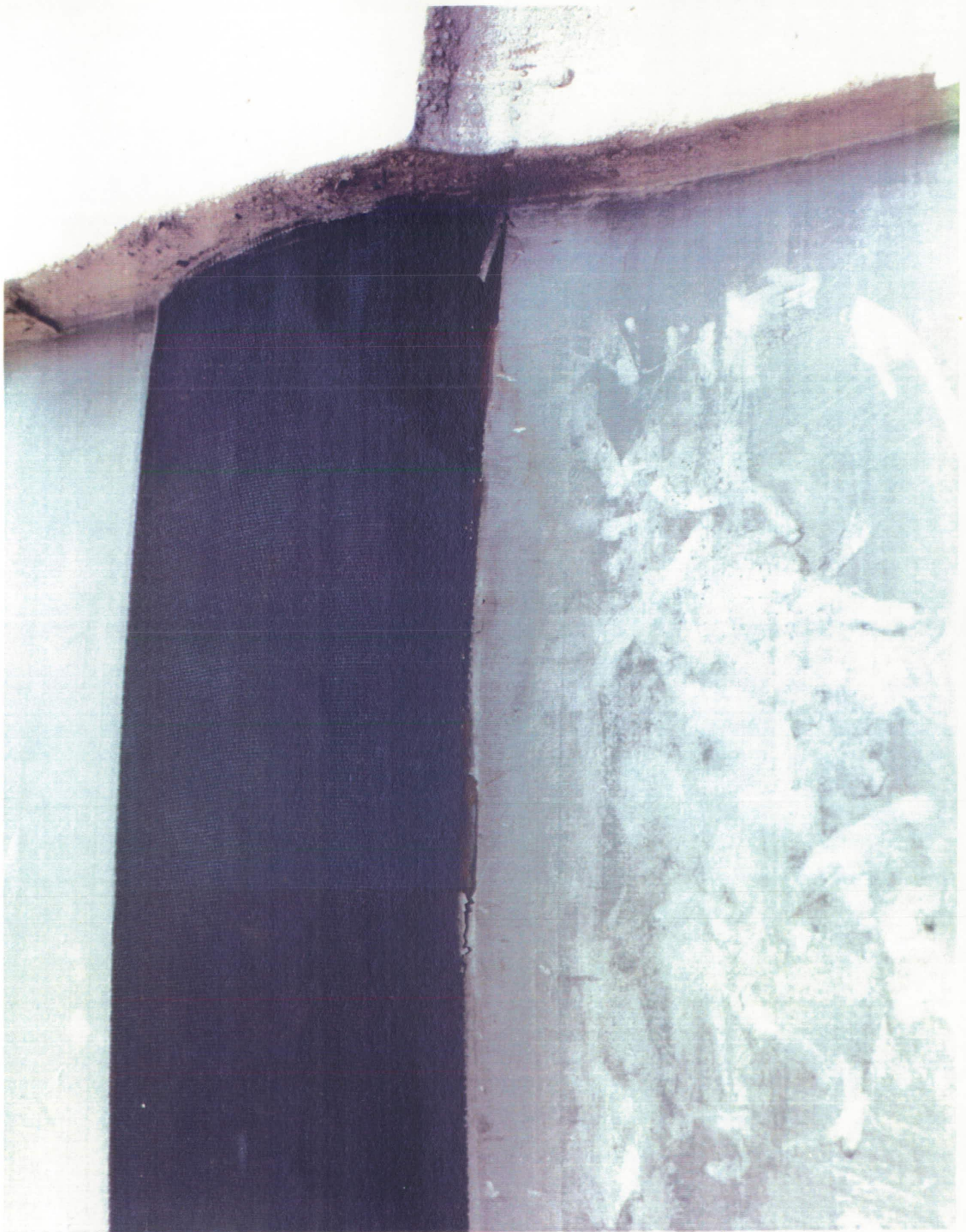
A 9.6-inch unbond occurred on the aft edge of the RFC factory joint weather seal
