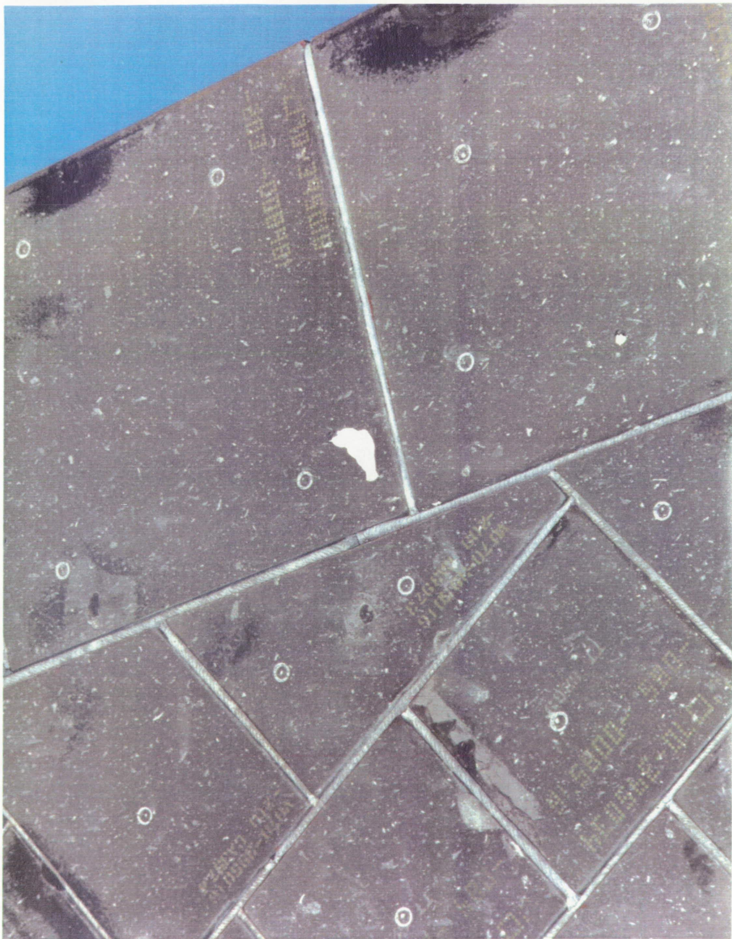
Typical tile damage from a debris impact on the body flap
