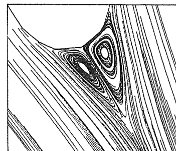
h) Particle traces near the trailing edge
