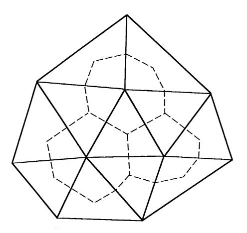
Fig. A3. Dual cells for rectangular and triangular grids
