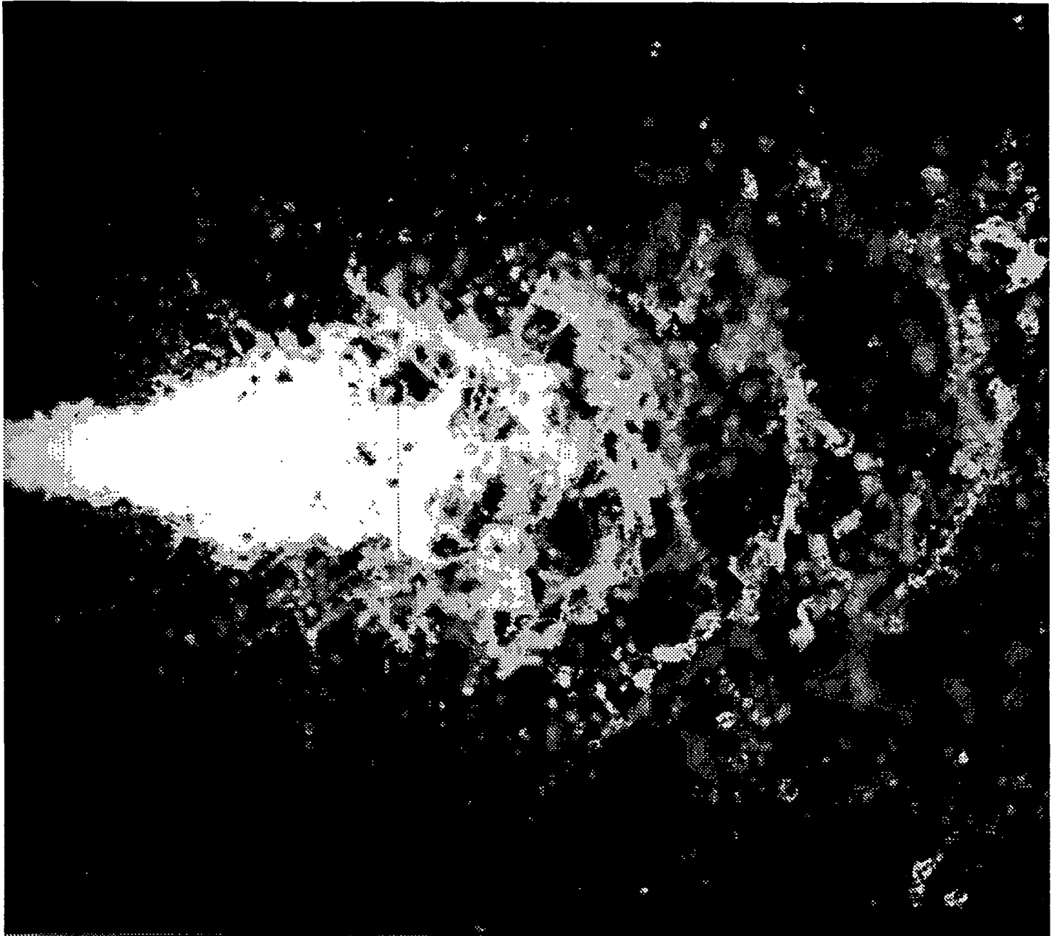
Figure 2.5 Close-up (enlarged) view of the point of impingement ( v=23.5 m/s, Re_D=46,300 , angle of impingement= 75^\circ ).
